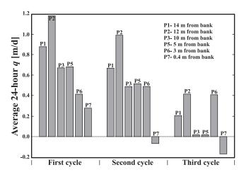
**Figure 3.** The average vertical flux over each 24 h cycle observed at each piezometer. P1 is the piezometer nearest to the middle of the river, while P7 is the piezometer closest to the bank. Average flux near the center of the river is always positive, while the average flux near the bank can be close to zero or negative.
