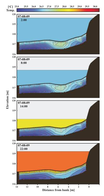
**Figure 8.** Temperatures in both the river and streambed. During low stage, the river's temperature signal penetrates deeper into the streambed. During upwelling, the temperature signal is confined to the uppermost 10 cm of the streambed.
