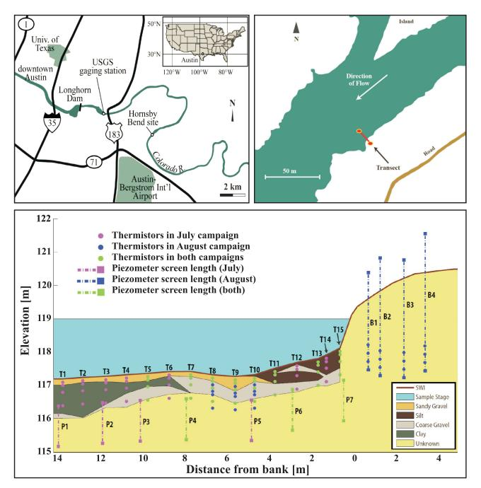
**Figure 1.** (top) Location of the field site, Hornsby Bend, on the Colorado River in relation to Austin, Texas landmarks and location of transect instrumented at Hornsby Bend (modified from *Sawyer et al.* [2009]). (bottom) Interpreted sediment distribution at the study transect estimated by probing with rebar to a maximum depth of 1.2 m, and placement of instrumentation in both field campaigns. The beige-colored "Unknown" sediments are most likely similar alluvial deposits.
