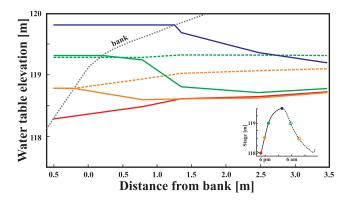
**Figure 7.** Bank water table profiles. The envelope of fluctuations implies that transient bank storage is at work and in fact may cause the hysteresis in streambed instantaneous flux near the bank (Figure 5).
