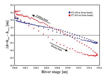
**Figure 6.** Head difference  $\Delta h$  between a streambed piezometer and the river plotted against river stage through a 24 h cycle. The relationship at P3, a piezometer 10 m from the bank, shows no hysteresis. While at P7, the piezometer located only 0.4 m from the bank, shows significant hysteresis. See Figure 1 for location of piezometers.
