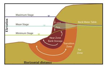
**Figure 10.** Conceptual illustration of effects of transient bank storage on hyporheic processes in the streambed adjacent to the bank. Transient bank storage is suggested as the cause for the hysteretic response seen in streambed fluxes at the bank. With increasing distance into the bank, this envelope of high impact bank storage dissipates.
