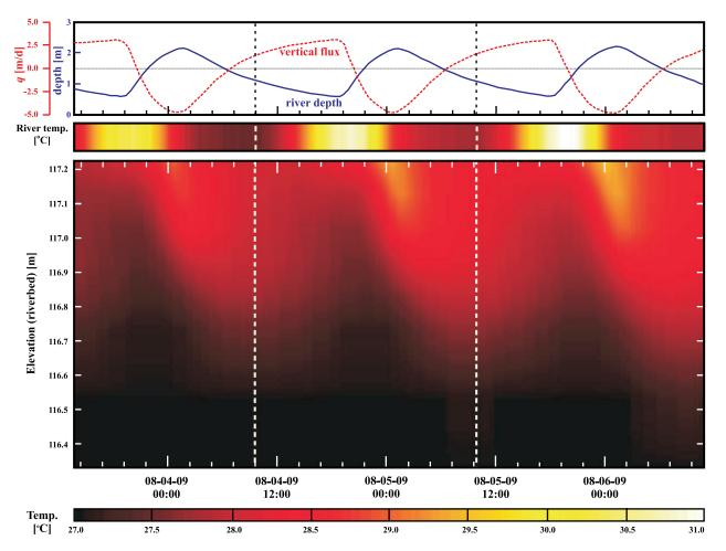
**Figure 9.** Streambed temperature, river temperature, river stage, and instantaneous vertical fluid flux through time at profile T10 in the transect (see Figure 1 for location). Positive flux indicates upwelling, while negative flux is downwelling. The top of the streambed temperature plot corresponds to the sediment-water interface.
