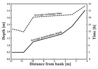
**Figure 4.** Depth of the hyporheic zone and exchange time calculated using vertical exchange fluxes. With increased proximity to the bank, both the extent of the hyporheic zone and the exchange time increases.
