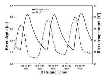
**Figure 2.** Observed asynchrony between river stage and temperature measured at Hornsby Bend over multiple 24 h cycles. Stage varies by 1.5 m with a mean depth of 1.3 m and temperature varies by approximately 3 °C each day.
