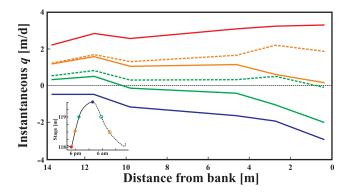
**Figure 5.** Spatiotemporal variation of instantaneous flux across the transect. When the river is at its lowest stage (red), the entire transect is gaining. When at maximum stage (purple), the entire transect is losing. The greatest variability in flux occurs at the bank. The inner framed key shows river stage over 1 day. Points indicate times when vertical fluxes are plotted in the graph. Solid lines represent rising stage while dashed lines represent falling stage.
